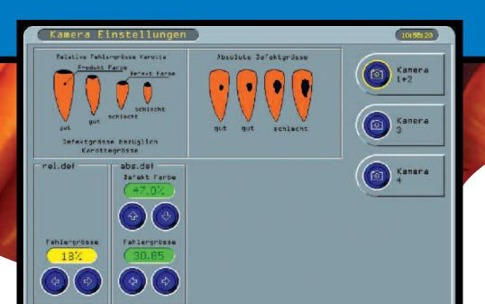
By means of a colour touch screen the MT<sup>®</sup> inspector is easy to operate and settings can be stored in a programme.
