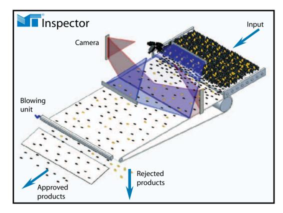
In this way the cameras will identify the bad spots and foreign components by means of colour recognition and the computers will control the blowing unit for the removal of the rejected carrots from the product flow.
