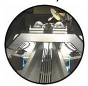
Originally the Ciris® was designed for round products such as potatoes, but it has also proved to be highly suitable for detecting undesirable products among mussels as well as barnacles and other organisms growing on mussel shells.
